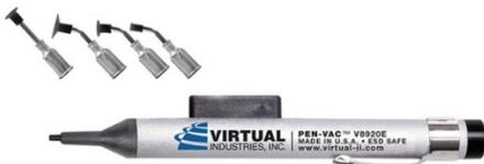
**V8920E-A-B** PEN-VAC™ JUNIOR, ESD safe, 5" X 1/2" aluminum body, kit with (3) bent probes with 1/8", 1/4" and 3/8" cups and (1) straight probe with 1/4" diameter static dissipative Buna-N rubber Black Vacuum Cups.
