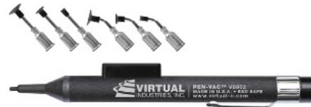
**V8902-LMS-B** Standard PEN-VAC™, ESD safe, 5 3/4" X 1/2" anodized aluminum body with storage compartment in the rear. Kit contains (3) bent and (3) straight probes with (2) each 1/8", 1/4", 3/8" diameter static dissipative Buna-N rubber Black Vacuum Cups.
